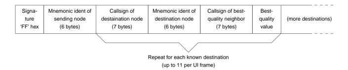
Up to eleven destinations are packed into each UI-frame, and the node broadcasts as many such frames as required to send its entire routing table.
